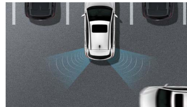
Rear Cross -Traffic Collision Warning When reversing out of a narrow parking space, the Rear-Cross Traffic Collision Warning reduces the risk of a collision. Using 2 radar sensors at the rear, it warns you in case of any approaching cross traffic.
