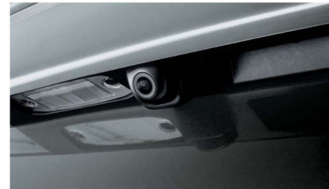
Rear-view camera The rear-view camera ends all worries about what could be hidden behind you like a parking bollard or a playing child. Shifting into reverse gear activates the rear-view camera allowing you to back-up with total confidence.
