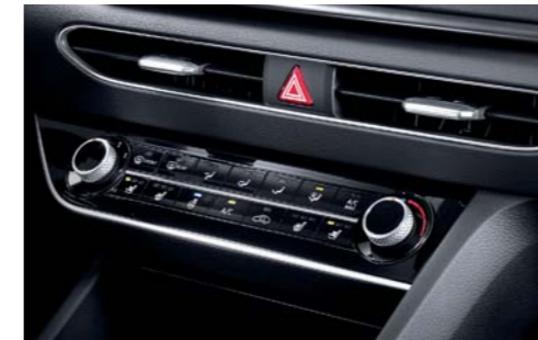
Manual air conditioning system
